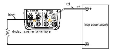
Figure 8 4-20 mA simulate transmitter source
