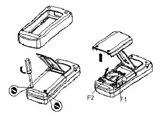
Figure 22 Replacing batteries and fuses
