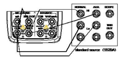
Figure 18 Adjusting all ranges of ohms
