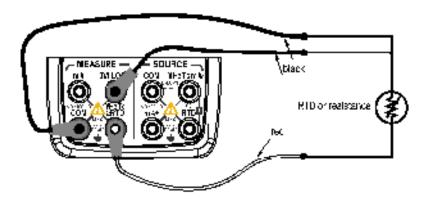
Figure 14 RTD signal with 3w method
