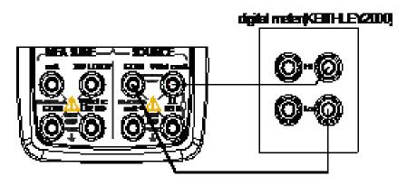
Figure 19 Adjusting voltage source
