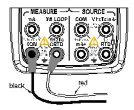
Figure 12 Measuring DC current
