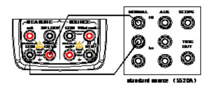
Figure 16 Calibrating DC voltage and frequency
