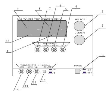
(1)Power switch: the unit is ON when this button switch is depressed
