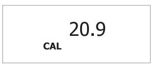
5) Press the "Enter Button ", the Display value will count from 30 to 0, then return to normal measuring screen and finish the calibration procedures. The complete calibration procedures will take 30 seconds approximately.
