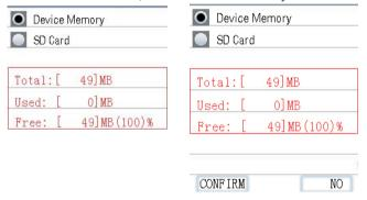
Press the ENTER button to format the flash or SD card, press ▲ button to cancel format, press ▼ button to confirm format.
