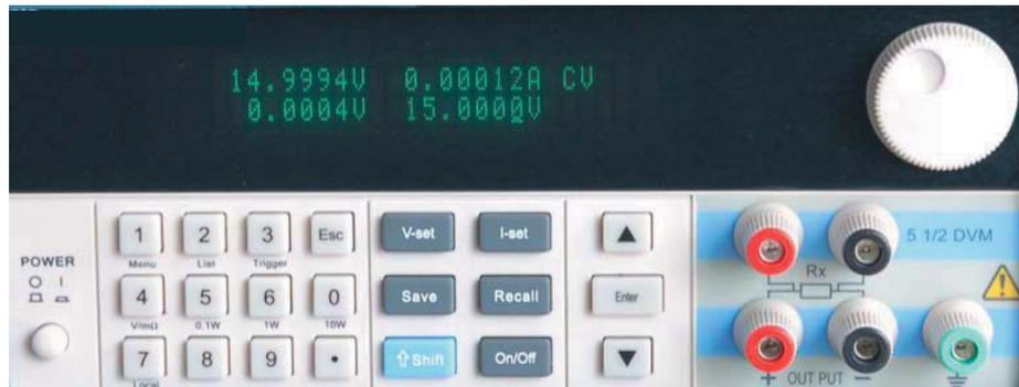
Diagram 3.1 the Front Panel of Power Supply
