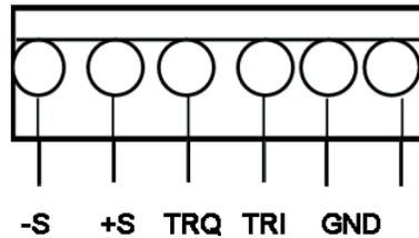
Diagram 4.4 Remote Measurement Terminals
