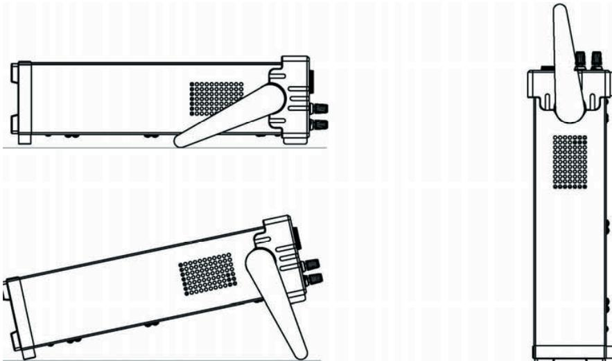
Diagram 3.3 Power Supply Viewing Positions
