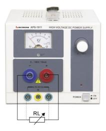
Load is connected as shown above. After the unit is switched on, output voltage indicated by Analoge meter (1). The instrument can supply Max.10000VDC
