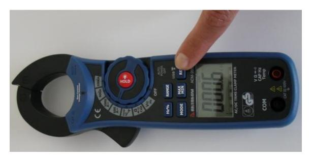
Please press REL button for 2 seconds to turn on the Wireless USB function, the icon appears on the LCD. When you have finish press the button again to return to normal operation.
