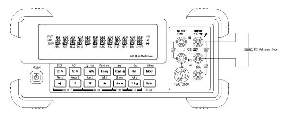
Input Resistance =  $10M\Omega$  on 1000V and 100V ranges; >  $10G\Omega$  on 10V, 1V and 100mV ranges
