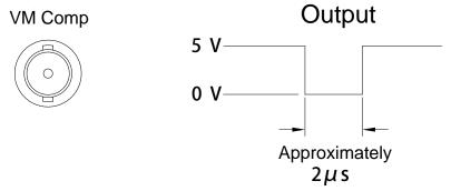
Figure 4-4 Trigger model
