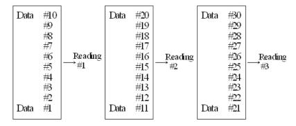
Figure 4-1 Moving average and repeating average filters
