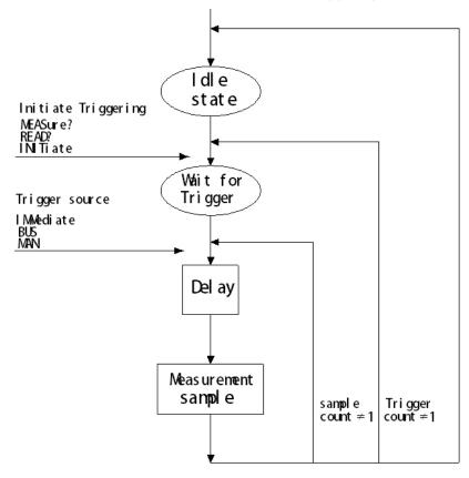
Figure 4-2 Trigger model
