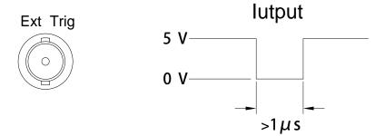
Figure 4-3 Trigger model
