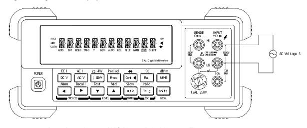
Input Impedance =1M $\Omega$  in parallel with <100pF
