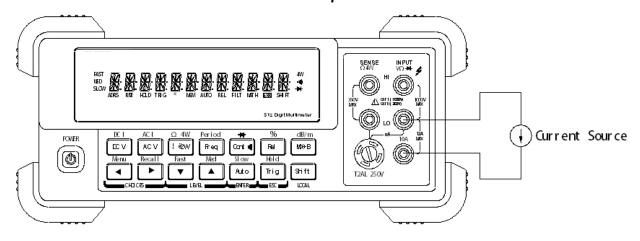
CAUTION: Maximum Input = 12A DC or RMS Figure 3-2 DC and AC Current Measurements
