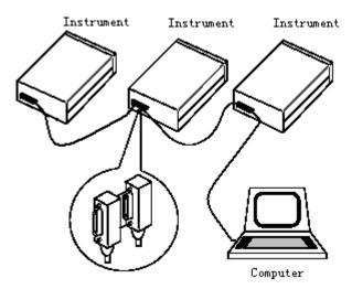
Figure 5-4 Typical GPIB System Interconnection
