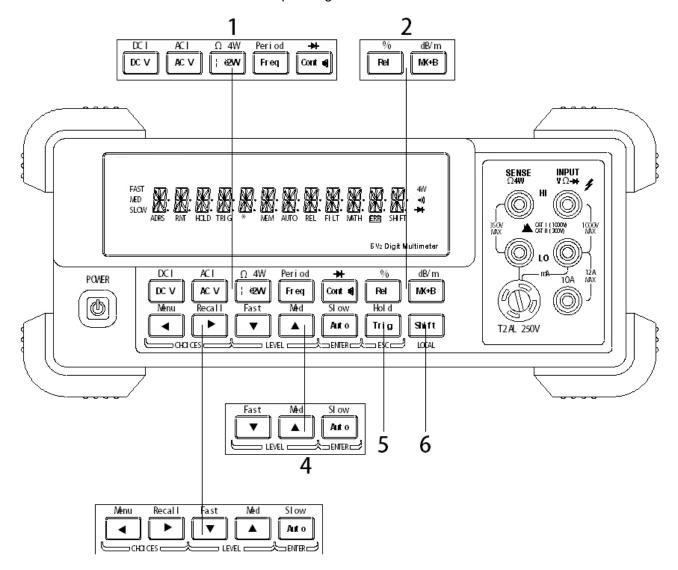
Figure 2-1 DMM Front Panel
